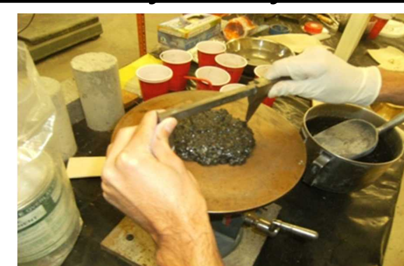
Figure 6. Flowability test performed according to ASTM C1437 and ASTM C1611 standards.
