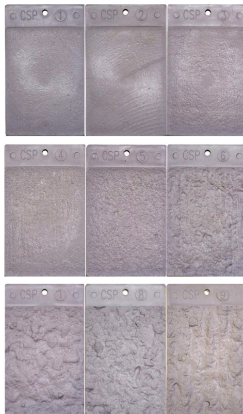
Figure 3-16: ICRI's standard CSPs
