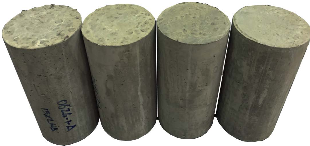
Figure 3-15: From left to right, concrete cylinders with 15%, 10%, 5% and no-LWA substitution.
