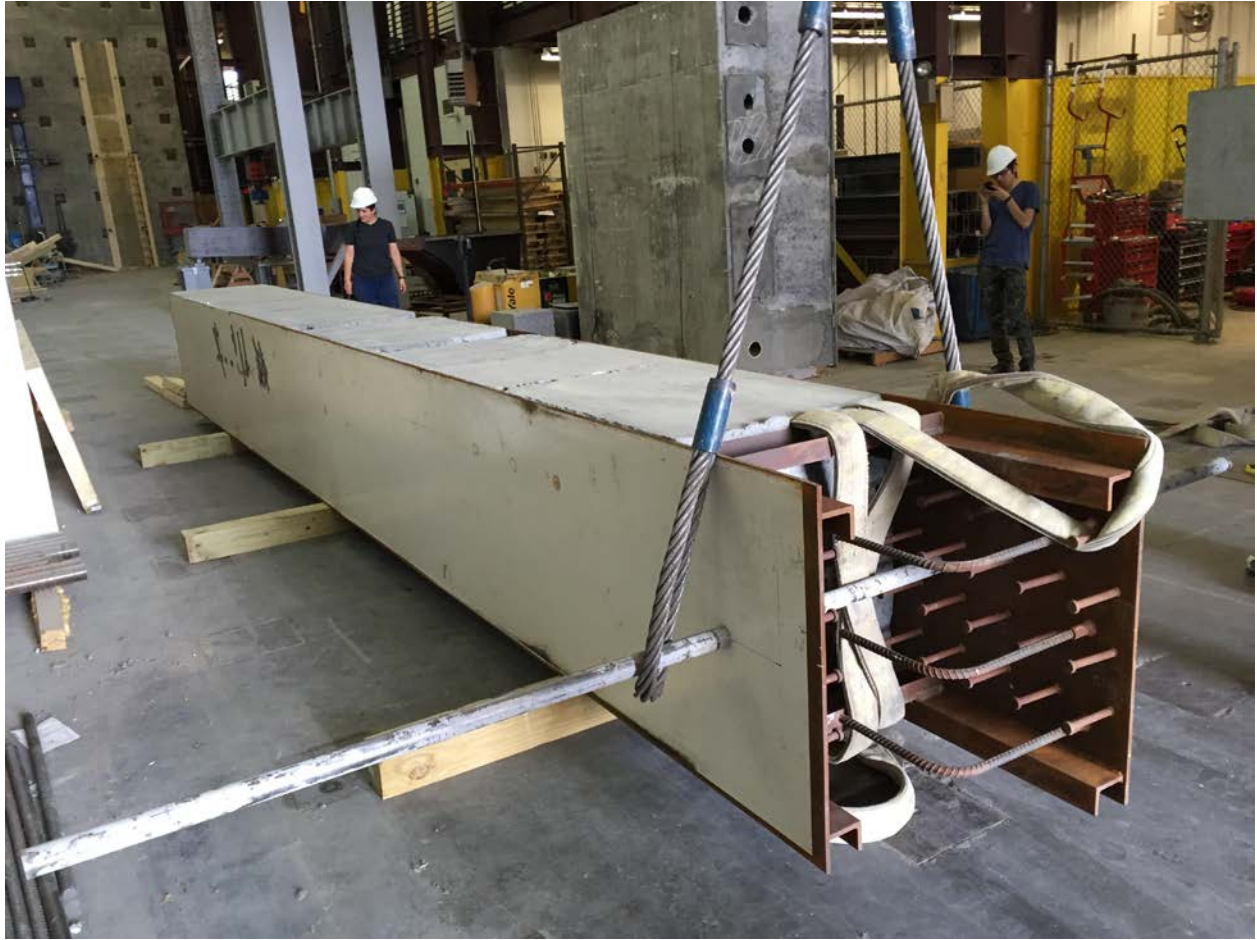
Figure 6-6. CA-20 module rotated into the horizontal position.
