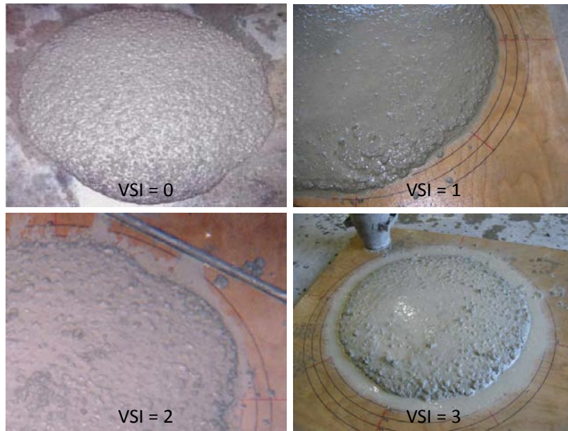
Figure 3-10: Visual stability index examples for various slump flow test
