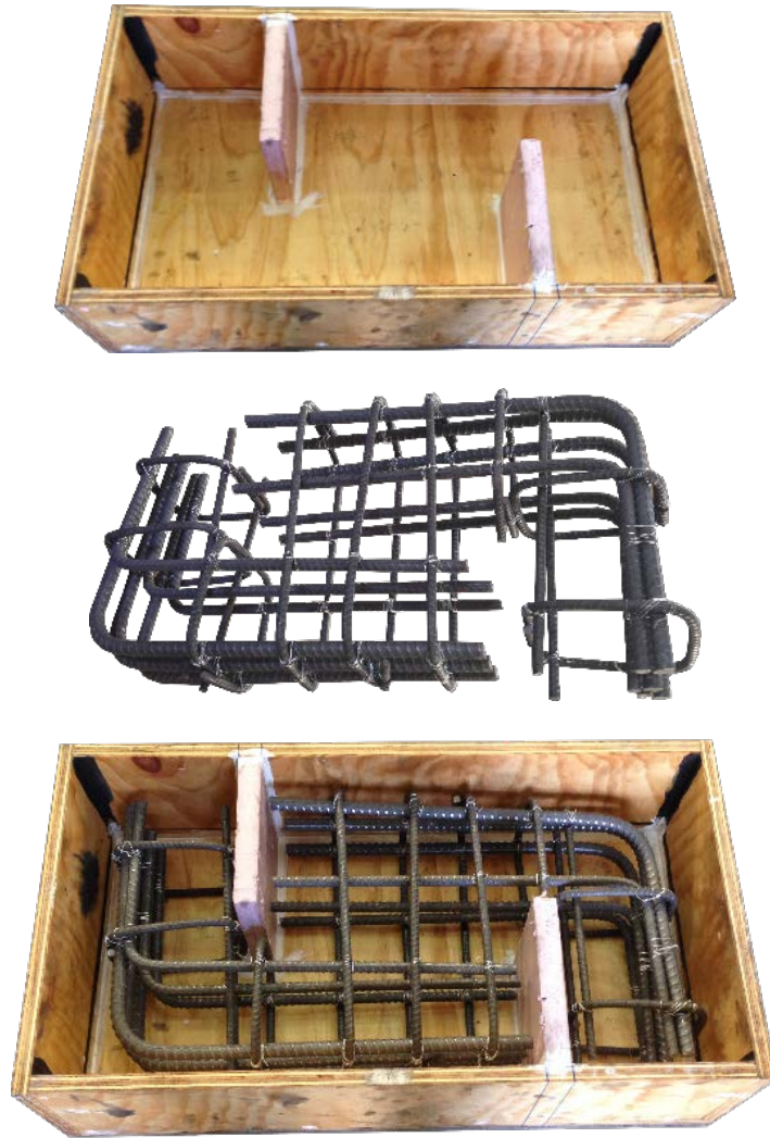
Figure 4-7: Monolithic Specimen Prior to Casting
