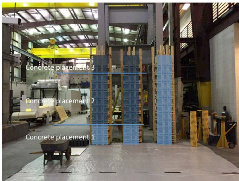
Figure 5-6. Concrete placement for Task 3 specimens.
