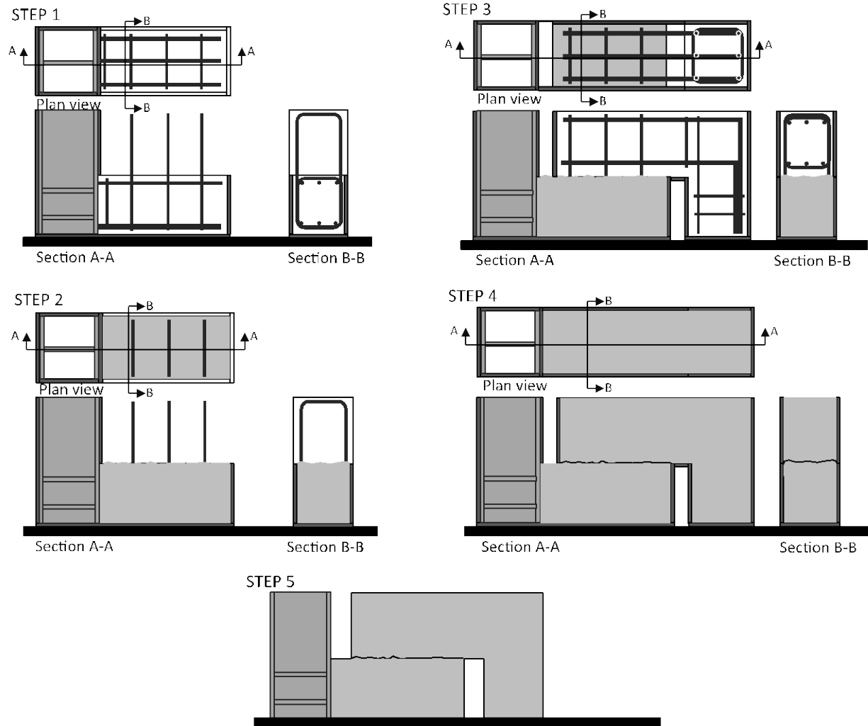
Figure 4-8: Steps for the fabrication of the shear friction specimens. The steps will remain the same for both steel reinforcement configurations. Step 1: Bottom mold with surface up. Step 2: Pour concrete in first part (day 1). Step 3: Add additional mold. Step 4: Pour concrete second part (day 2). Step 5: Cure 28 days
