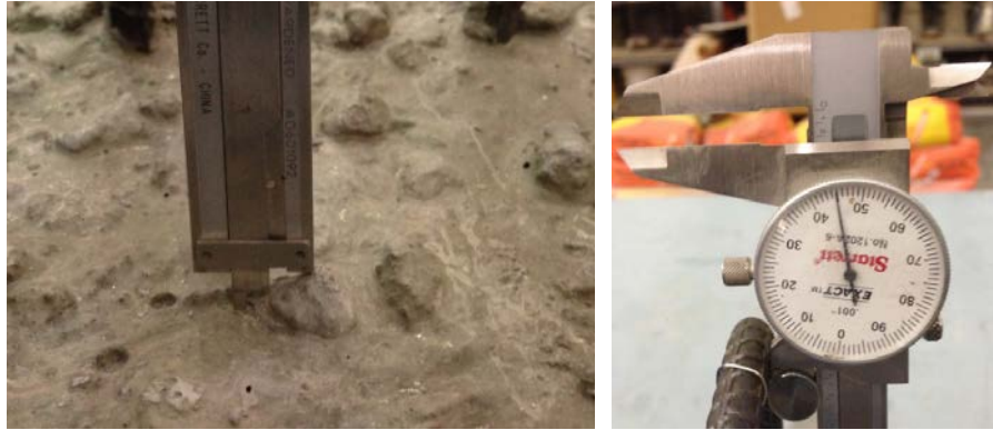
Figure 3-17: Roughness quantitative measurements
