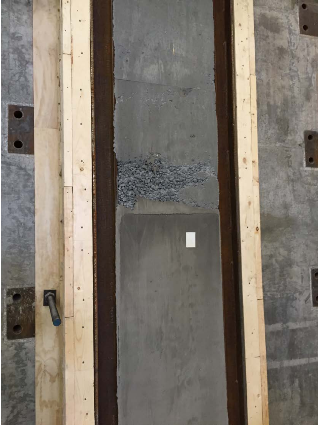
Figure 6-7. Segregation in SCC due to excessive slump.
