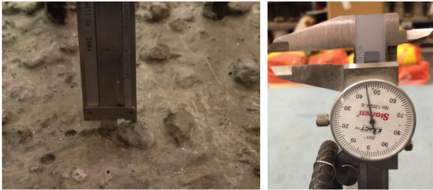
Figure 3: Roughness quantitative measurements.
