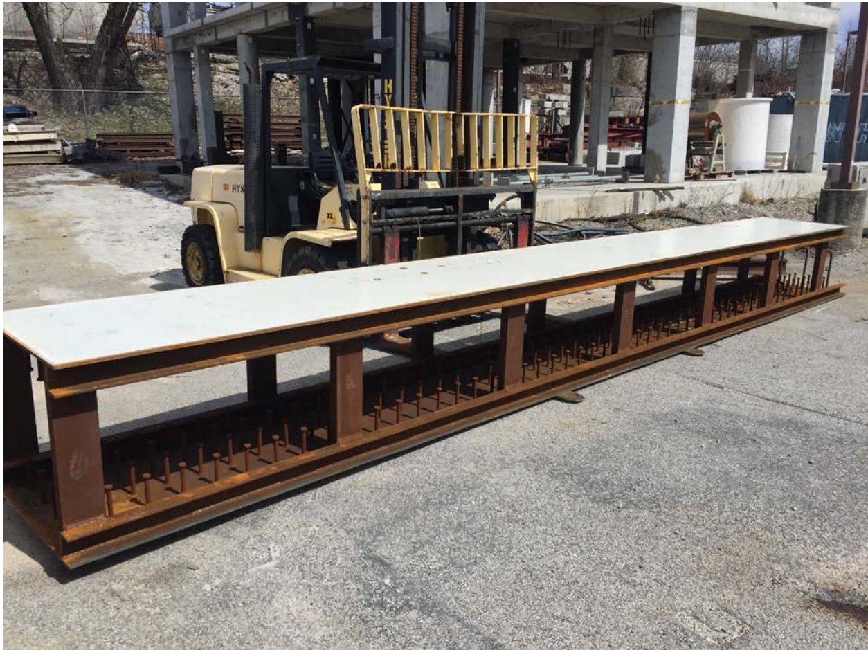
Figure 6-2: CA20 module section as received from Westinghouse.
