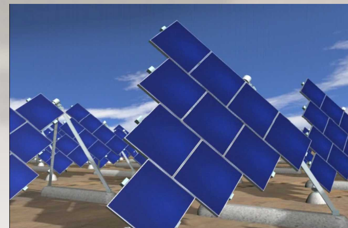
Conceptual vision of the system of flat concentrators mounted on inexpensive trackers.
