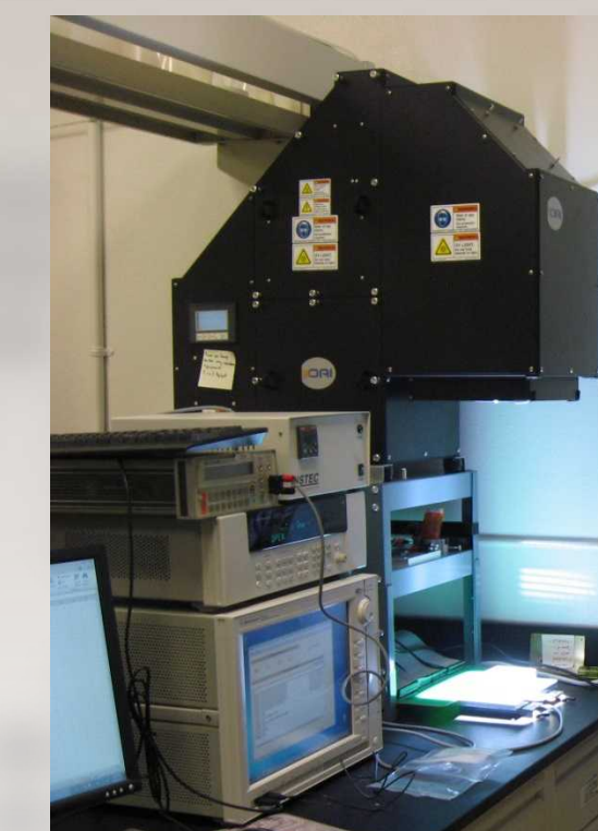
OAI Class AAA solar simulator and Agilent B1500 used for indoor testing
