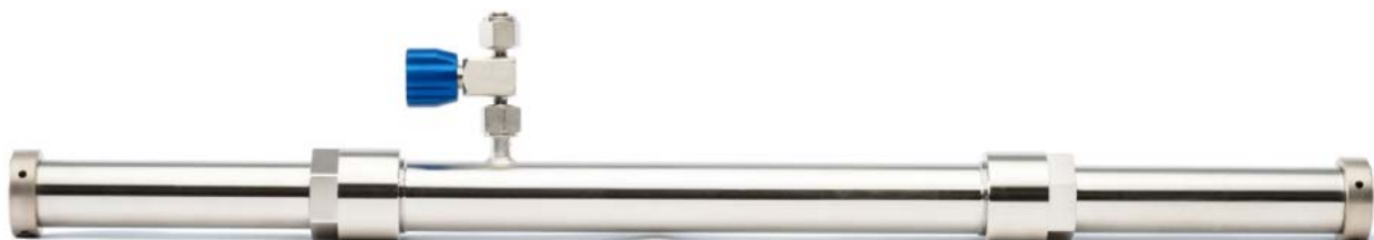
Figure 4. ^4\text{He} detector for used fuel storage monitoring using neutron fingerprinting.
