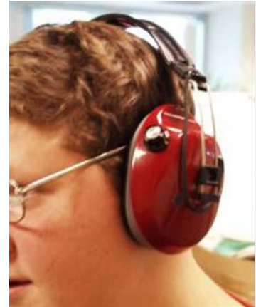
The seal between the ear cups and the user's head ( above ) may be affected by eyeglass temples, face shields, respirators, or long hair.
