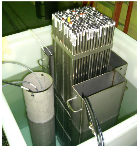
Figure 8 Mock-up fuel assembly in the center of the water tank surrounded by detector and neutron generator pods
