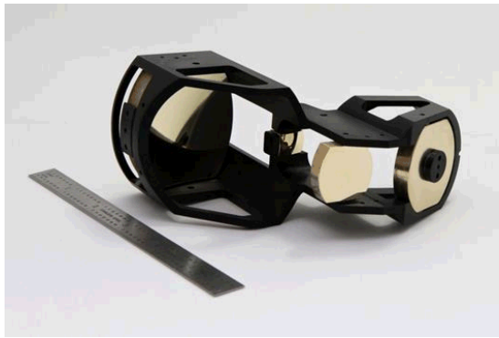
Figure 7. Full monocular prototype. Right image includes cover used to eliminate stray light during viewing.
