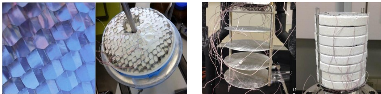
Fig 3.0(1): Photographs of the two prototype hydrogen storage systems. (Left) Hex-cell prototype, showing magnified view of hexagonal-cells of the heat exchanging manifold and top-view of the manifold filled with MOF-5 powder. The vertical rod in the center of the manifold is the resistive heating element. (Right) MATI prototype, showing the empty manifold and the manifold loaded with 8 MOF-5 pucks.
