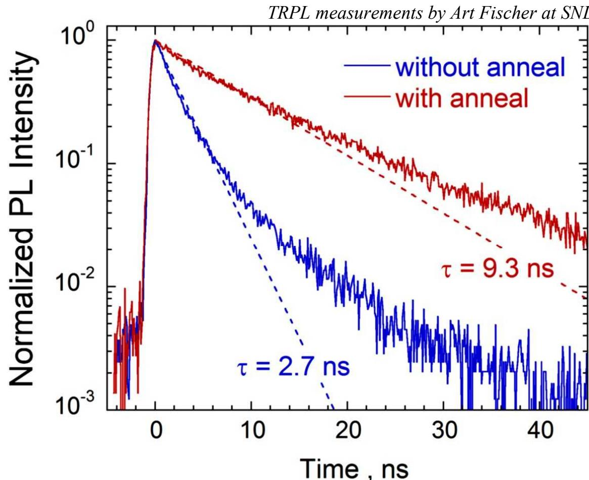
Annealed AlGaN/InGaN layer has longer lifetime than without anneal.
