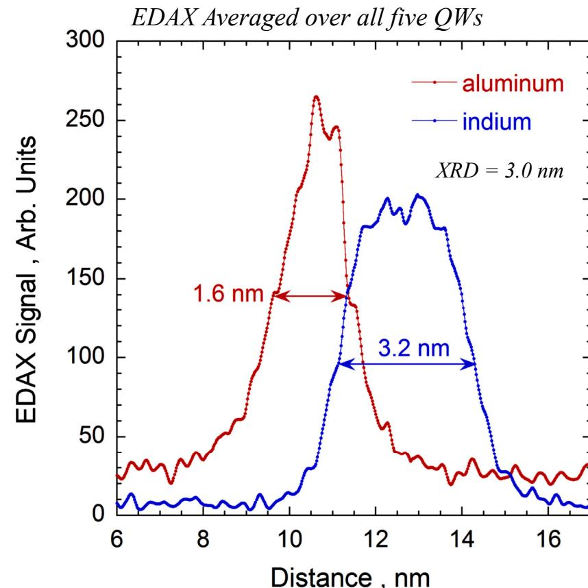
Top and bottom InGaN interfaces are both  $\sim 1$  nm thick.
