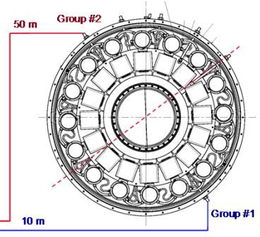
**Experimental device :** the trigger circuit of a LTD cavity has been separated in 2 circuits in order to trig separately two groups of 8 bricks
