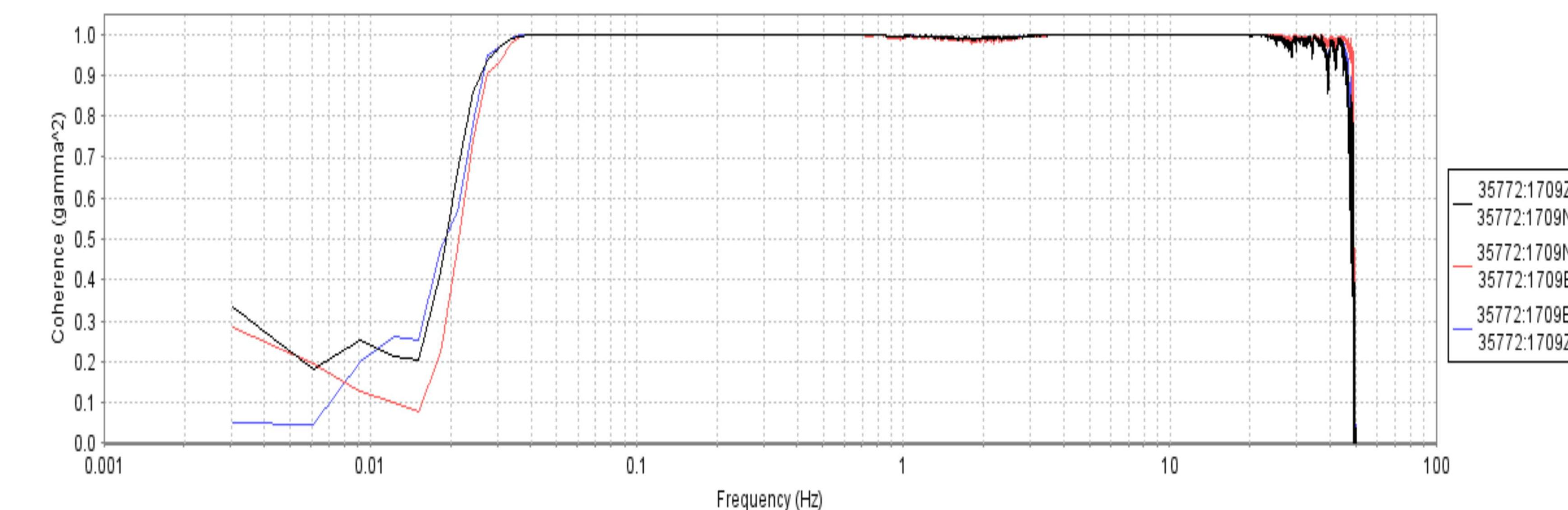
The coherence improves even more when all three sensors are thermally insulated. The coherent band widens from 0.04 to 30 Hz.
