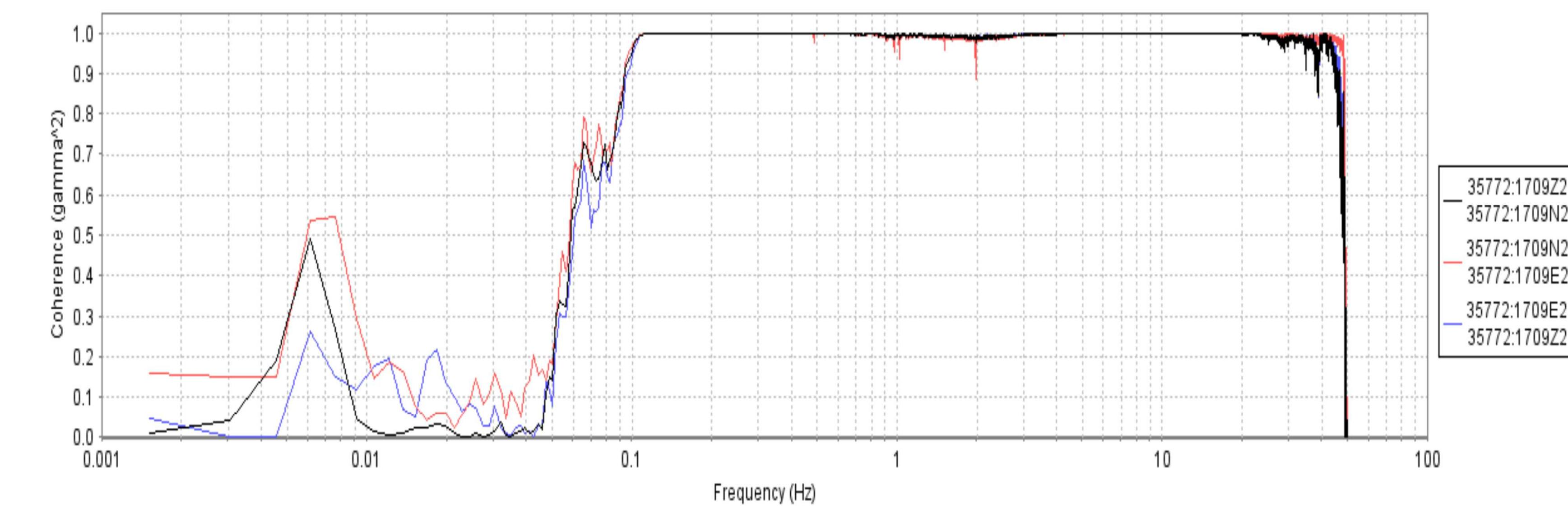
The coherence improves significantly after the three sensors are fine aligned with a deviation from the N-direction of less than one degree.
