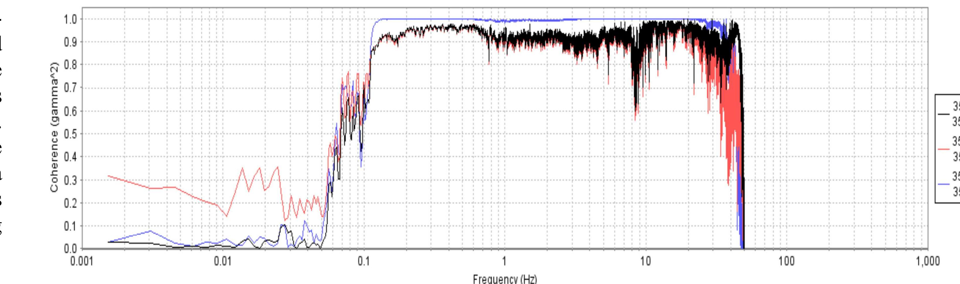
A rough alignment of the three sensors within a few degrees leads to poor coherence over the whole frequency band.
