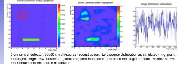
3 cm ring source; 36000 s multi-source reconstruction. Left: source distribution as simulated (ring, rectangle). Right: raw "observed" (simulated) time modulation pattern on the single detector. Middle: MLEM reconstruction of the source distribution.
