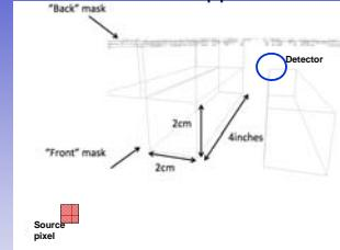
For each source pixel and each mask rotation position, build probabilities of detection by integrating attenuation of mask over possible particle trajectories. Accounts for imperfect opacity and finite pixel/detector size, but not scattering.
