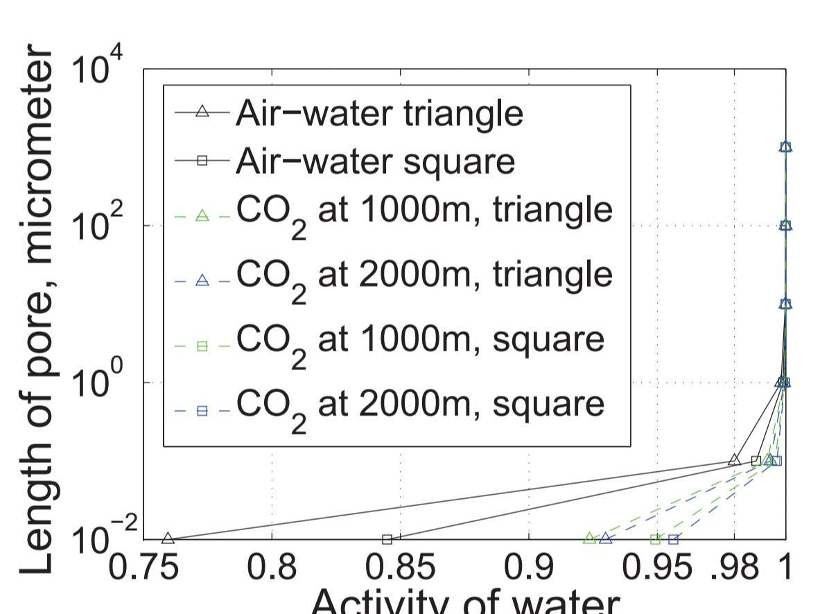
Assuming that the chemical potential of the pore-scale model can be related to that of EQ3/6 through  $\Delta\mu = RT\ln(a_{H2O})$ , the plot of Part III is reproduced here. The possible conclusion is that snap off may not occur for large pores in the CO<sub>2</sub>-water system since high activities of water may not be reached.
