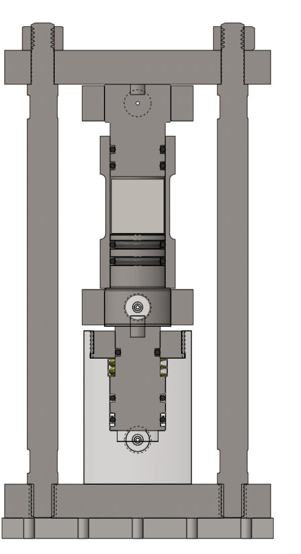
Ongoing work: capillary condensation will be tested at the neutron beam facility at LANL-LANSCE. The experiments to be performed in Feb. 2013 included measurement of pore structure of a swelling clay before and after wet scCO<sub>2</sub> flows through a constant volume oedometer (unxial state of stress).
