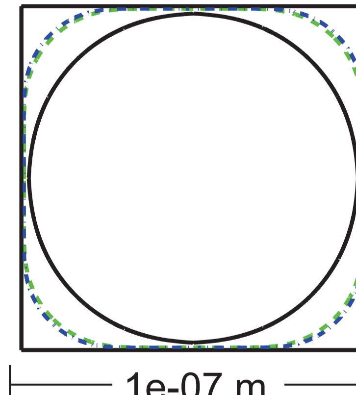
Chemical potential for air-water "snap off" in triangular pore is -2,786 J/kg. The CO<sub>2</sub>-water interfaces for the same chemical potential in much reduced saturation (percent of pore space filled with water).
