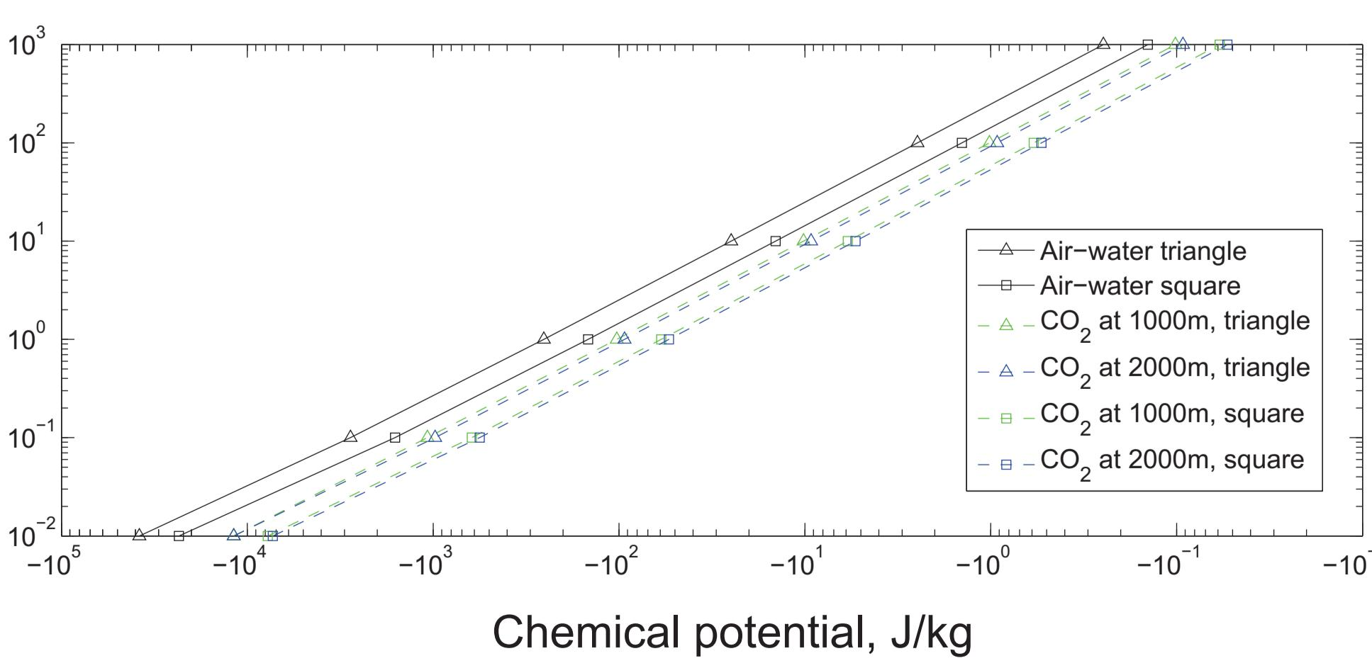
**"Snap off" for a given pore size vs. chemical potential:** the figure to the left shows the chemical potential at snap off in a pore of a given size (the length of a side for a triangle or square pore) for the air-water and CO<sub>2</sub>-water systems. The relationship is linear in log-log space. At a given pore size, snap off for the CO<sub>2</sub>-water system requires less negative chemical potentials (e.g., greater water activity).
