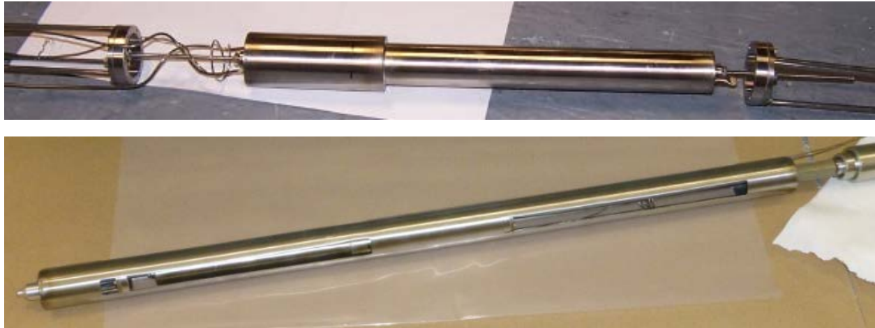
Fig. 3. “Fuel rod” thermoacoustic sensor. (Above) The thermoacoustic resonator is shown at the center of the photograph. The resonator tube has an inside diameter of 2.2 cm and is 22 cm long. The hot section of the resonator holds the hot heat exchanger that contains two enriched ^{235}\text{U} fuel pellets that are each approximately 5 mm in diameter and 10 mm long, as well as the extruded ceramic “stack.” The hot section is surrounded by an insulation tube with an outside diameter of 3.0 cm, which is about 7.5 cm long, containing a \text{SiO}_2 floss. That insulation space is filled with air at atmospheric pressure. The remainder of the resonator tube is empty other than containing the 2.0 MPa mixture of 75% He and 25% Ar that fills the entire resonator. The empty portion of the resonator has a 0.51 mm wall thickness and is in good thermal contact with the reactor’s coolant water. The two 4-40 threaded rods that extend from either end of the resonator are attached to two circular stainless steel (SS) disks that are 200 microns thick and have six spokes that act as cantilever springs to allow the resonator to vibrate axially but constrain the resonator to remain coaxial within the surrounding “slotted tube.” The rings that clamp the periphery of the springs are each welded to three SS rods to facilitate insertion into the slotted tube after assembly. Exiting the insulation tube at the left are two Type-K thermocouple (T/C) leads. One of the thermocouples is silver-soldered (brazed) to the thin-walled section of the resonator next to the heat exchanger and the other is silver-soldered to the hot end of the resonator. Both T/Cs are located within the insulation space. A rhodium neutron flux sensor, with a sensing length of 9.8 cm, is coiled in the space between the end of the insulation tube and the adjacent spring. (Below) The resonator and springs are contained within a “slotted tube” that has the same outer diameter as the fuel rods. The slots allow the reactor’s coolant water to remove the heat of fission from the thermoacoustic sensor and facilitated testing of the resonator’s axial mobility before insertion in the reactor’s core.
