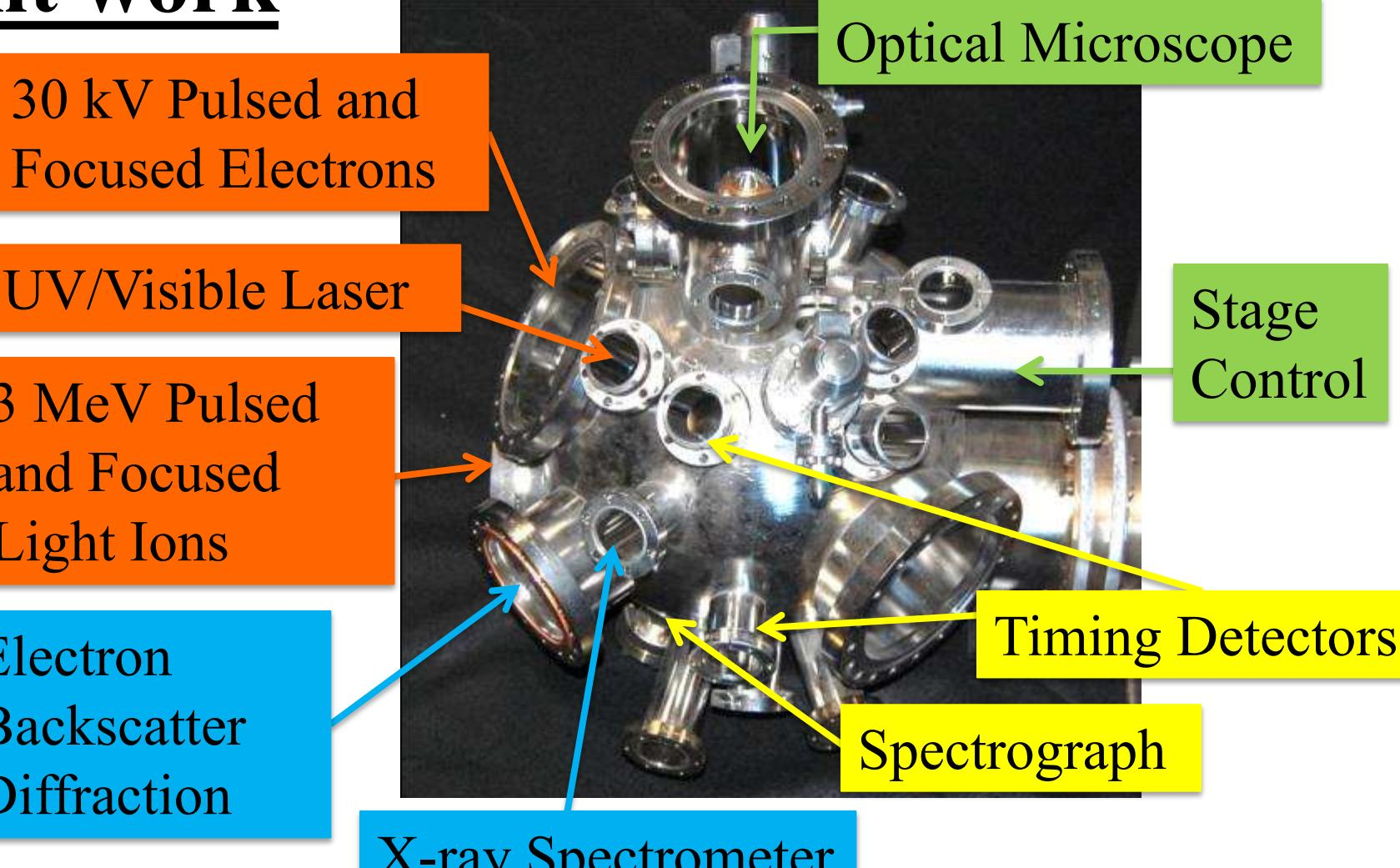
An optical port is currently being added to the I<sup>3</sup>TEM, which, if successful, will permit *in situ* TEM CL and IBIL
