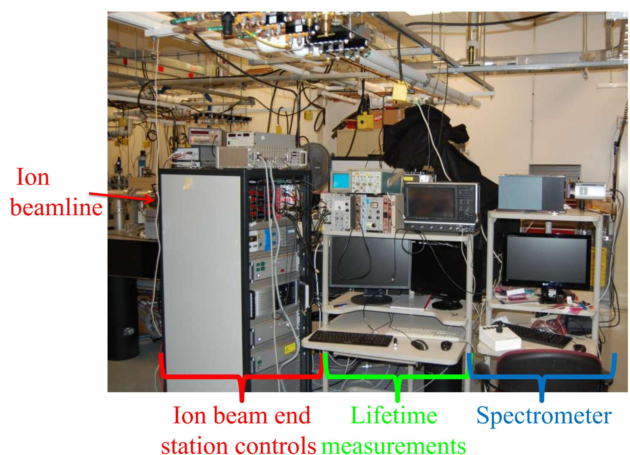
The Ion Beam Lab's microbeam end station on the 3 MeV Pelletron accelerator permits precise location of the irradiated regions, as well as IBIL spectra and lifetime measurements
