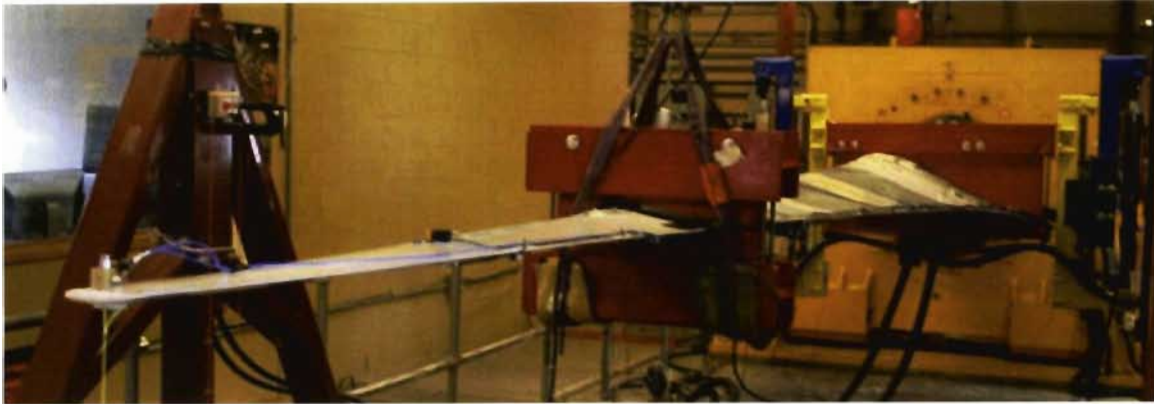
Figure 1. Test setup: a 9m CX-100 blade under a fixed-free condition
