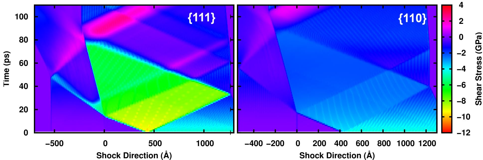
Stress required to nucleate voids in  $\{111\}$  and  $\{110\}$  interface is 8.8 and 8.5 GPa, respectively.
