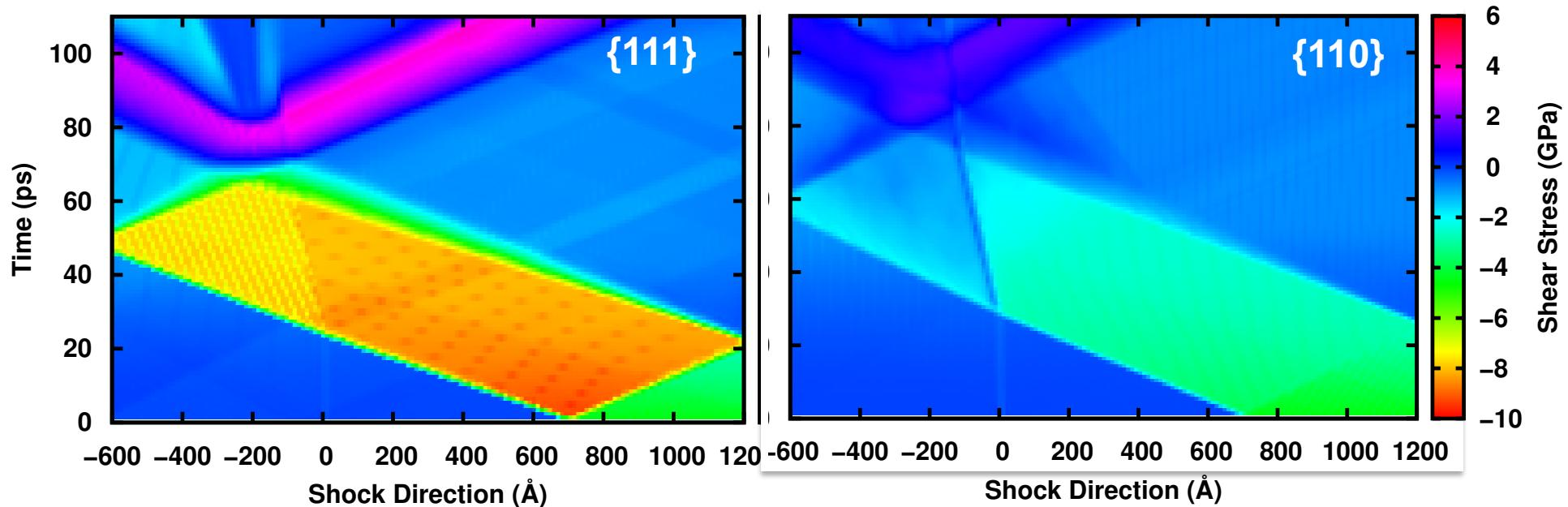
Stress required to nucleate voids in  $\{111\}$  and  $\{110\}$  interface is 11.3 and 10.4 GPa, respectively.
