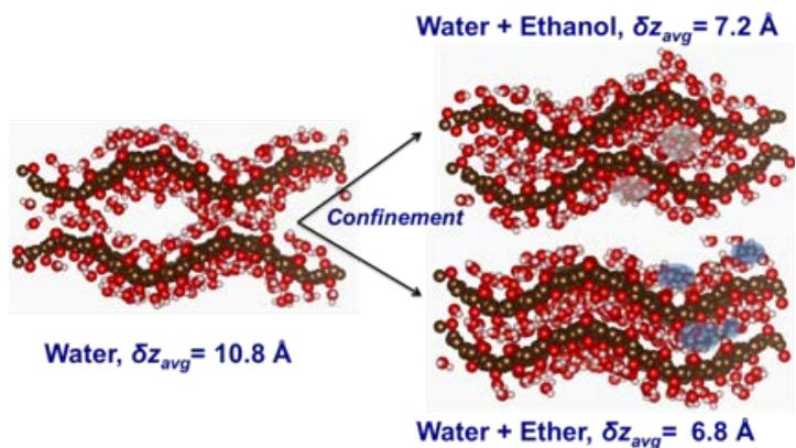
Theoretical models of solvent-treated graphene oxide structures. Molecular dynamics relaxed structures for water, water/ethanol, and water/ether. Brown spheres represent carbon atoms, red spheres represent oxygen atoms, and white spheres represent hydrogen atoms. Addition of solvent molecules in between each layer leads to a decrease in d-spacing as observed from XRD data.
