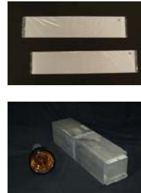
ZnS:Ag/6LiF screens allows identification of neutron capture
