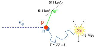
Standard detection of gammas and neutrons in coincidence
