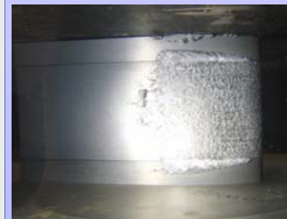
MHKF1-180s Sigma = 1.0 dist. roughness (60 grit)
