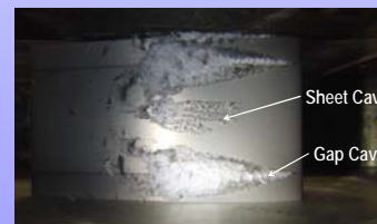
MHKF1-180s sigma = 1.1 alpha = 8 deg.
