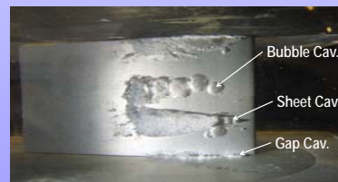
NACA 4412 sigma= 1.1 alpha = 8 deg.
