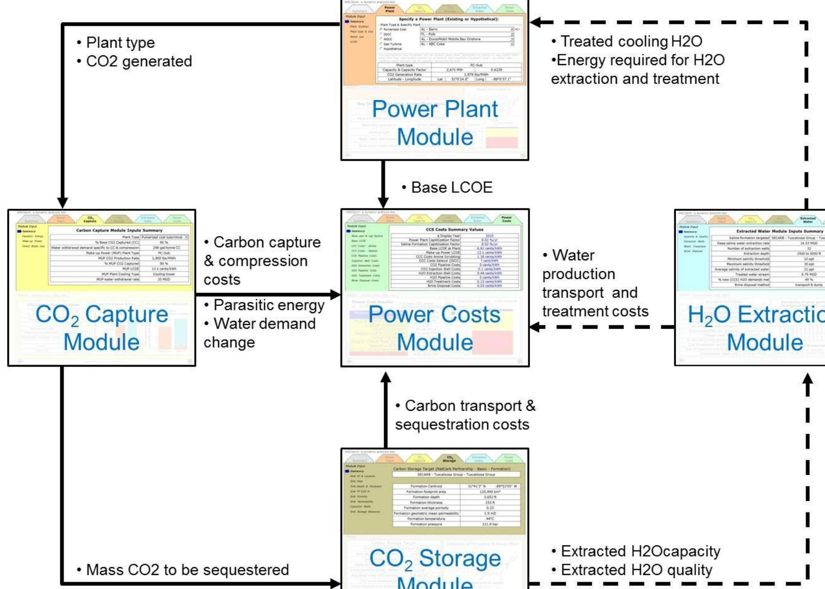
Sandia National Laboratories has developed the Water Energy and Carbon Sequestration simulation (WECSSim<sup>®</sup>) model to evaluate the costs and CO<sub>2</sub> amounts that would be associated with large scale CO<sub>2</sub> capture from any coal or gas fired power plant in the United States and permanent storage in the most economically viable deep saline formations. WECSSim evaluates the costs associated with removing saline water from the storage formation for pressure management.
