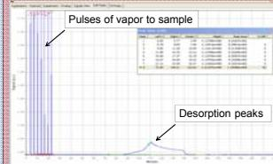
The pulse chemisorption experiment begins with a degas step to 600 °C. The sample is cooled to RT, then dosed with adsorbate until saturation, which is determined by a thermal conductivity (TCD) detector. The furnace then heats the sample at a specified ramp rate, and the desorbing gas is monitored. In these experiments, the samples were heated to 600 °C between 2 and 15 deg/min.
