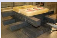
HDPE/paraffin cave used for neutron thermalization.
