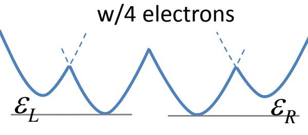
Exchange energy of right DQD =  $\begin{cases} J_R(|S\rangle) = E_{st} - E_{ss} & \text{when left dot is singlet} \\ J_R(|T\rangle) = E_{tt} - E_{ts} & \text{when left dot is triplet} \end{cases}$
