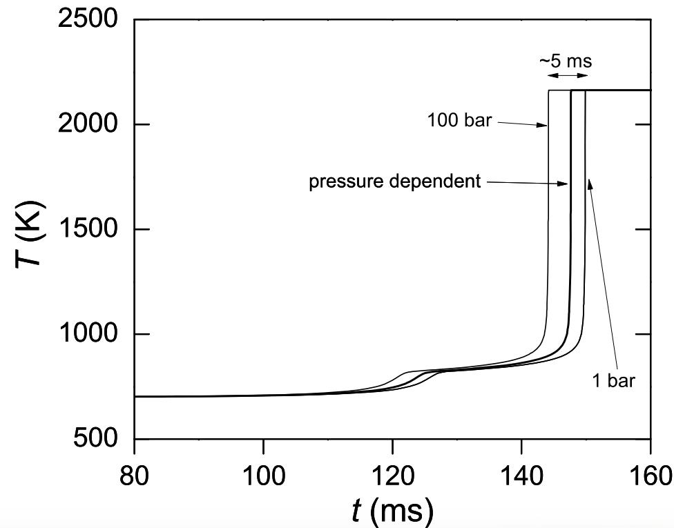
5 ms at 1200 rpm for example is equivalent to 36 degrees in crank angle, which is a significant fraction (1/10) of a stroke!
