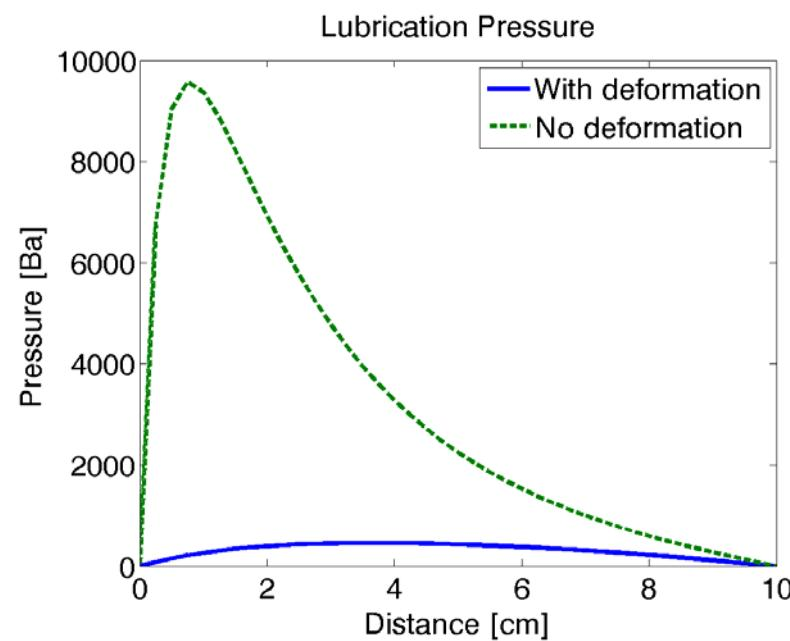
Lubrication pressure is greatly decreased when the slider is allowed to deform.
