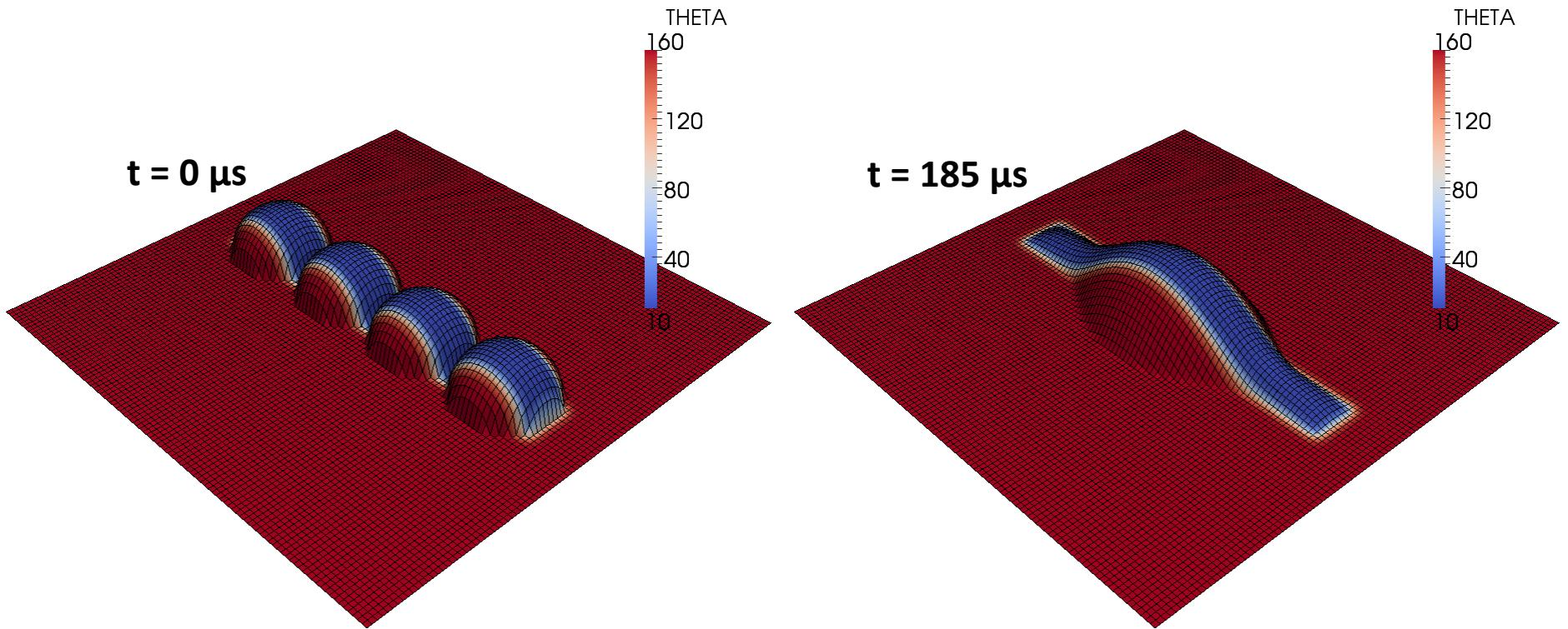
Resulting droplet does not conform to the pattern due to excess liquid deposited
