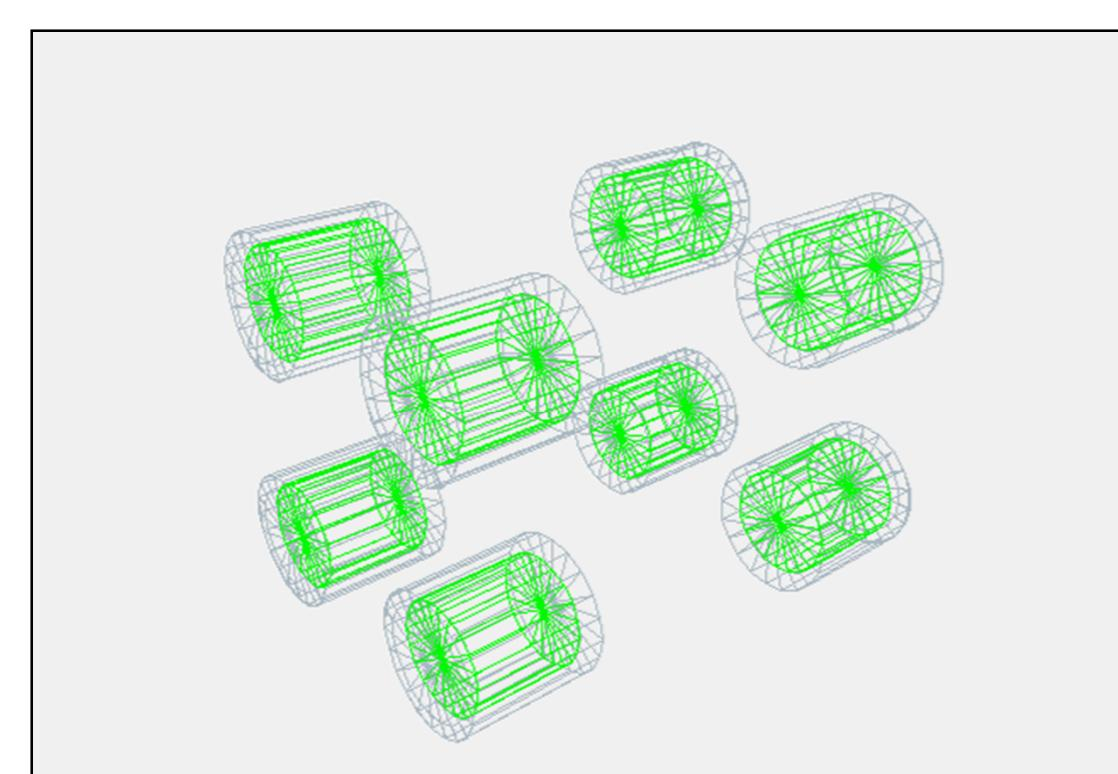
With a known forward source, the optimized 2" + 4" setup outperforms a uniform 3" + 3" configuration. However, without a known source location, there is an overall gain in efficiency moving to a uniform 3" thickness on both front and rear cells. There is also not a large degradation of image quality.
