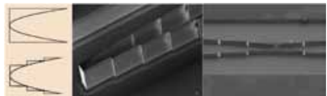
Left: A comparison of the solid refractive shape (top) with a kinoform shape (bottom). Middle: A parallel-to-point kinoform lens. Right: A point-to-point kinoform lens. ( Evans-Lutterodt et al., 2003 )
