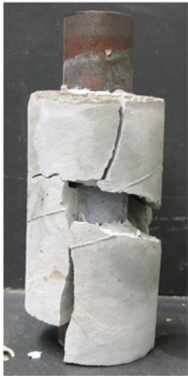
Conventional cement After 1 thermal shock cycle
