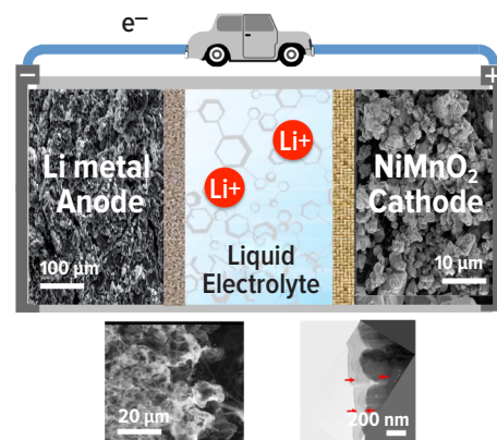
Figure 3-1. Heterogeneities, interfaces, and disorder are primary features of batteries. The Li-ion battery stores and releases energy by transferring \text{Li}^+ ions across interfaces among the anode, electrolyte, and cathode. The interfaces are not perfectly flat surfaces as often imagined in cartoons of the battery; instead, the electrodes are composed of grains that may range from nanometers to micrometers. Because of their small size, the interfaces of these grains are curved, thus exposing many atomic planes to the electrolyte, which in turn accelerates or retards specific side reactions. As \text{Li}^+ ions move through the interfaces, they expand or contract the surface, often leaving permanent strain or fractures in their wake. Each of these static and dynamic interface phenomena has the potential to help or harm the energy storage process. (Yu et al., 2015; Shi et al., 2015; Chang et al., 2015; Kim et al., 2015)
