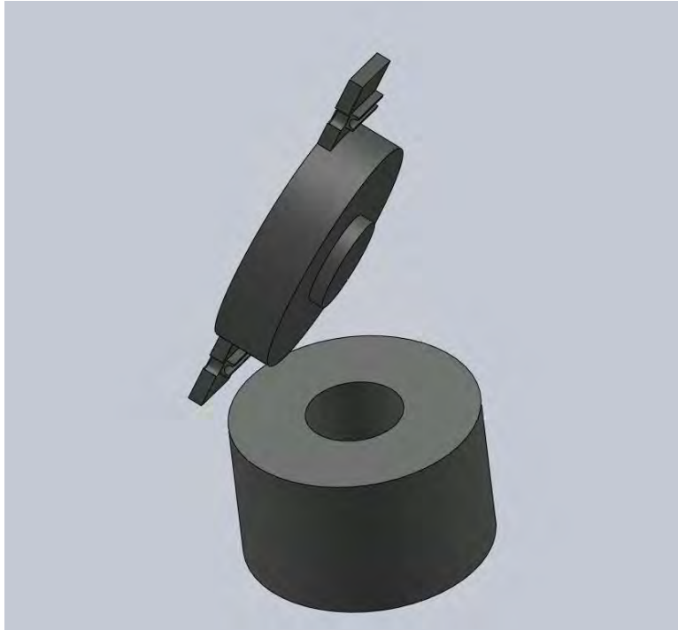
Figure 4.3. The lead container in which the target will be shielded completely.
