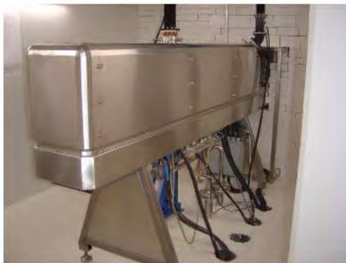
Figure 2.11. MEVEX accelerator used for the production of molybdenum-99. Also, these MEVEX accelerators can come in a clustered accelerator facility which can have up to four accelerators in one facility and is shown below in Figure 2.12 [12].
