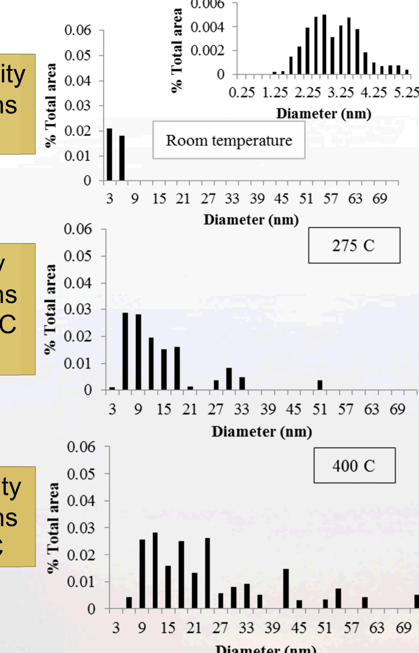
No preferential cavity growth along grain boundaries during annealing compared to bulk
