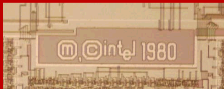
Die marking on same part has different manufacturer
