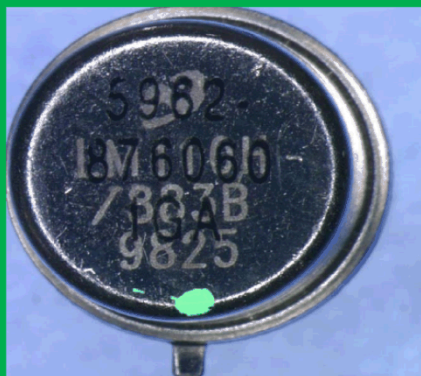
Laser etched markings have been stamped over with ink
