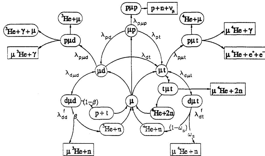
Simplified diagram of muonic processes in the TRIUMF solid hydrogen/deuterium/tritium target showing *observable states* and some parameters which *have been measured* or *will be measured*.
