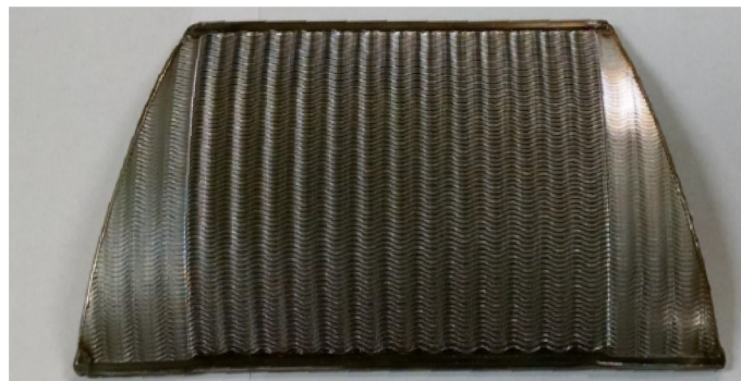
Figure 4. Folded, crushed and welded AFA F4 80μm foil air cell that was assembled into a C65 recuperator.
