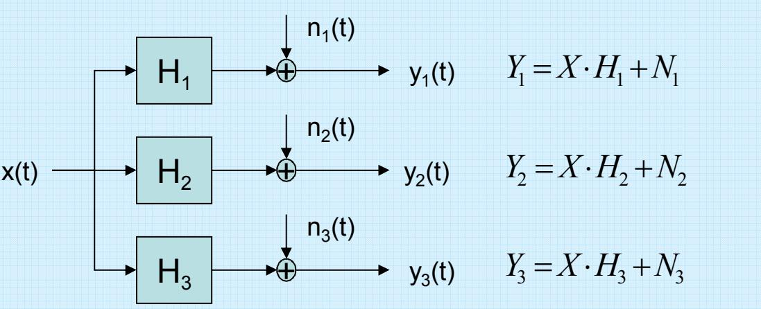
Given just the outputs  $Y_i$ , the cross-power spectrums  $P_{ij}$  can be computed. Given the assumptions that the channels are all measuring a common signal and the noise for each channel is independent, the cross-power spectrums can be used to estimate the noise power spectrum ( $N_{ij}$ ) and the channels' relative system response ( $H_j/H_k$ )
