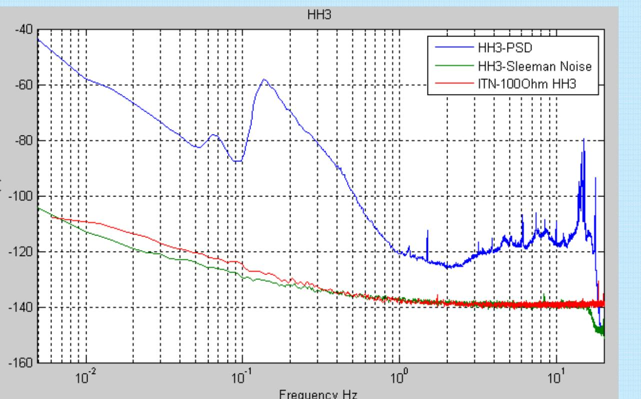
Approximately 71 dB of SNR for estimated coherent to incoherent energy from technique.
