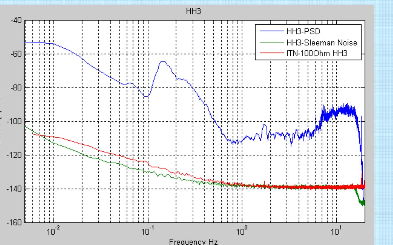
Approximately 72 dB of SNR for estimated coherent to incoherent energy from technique.
