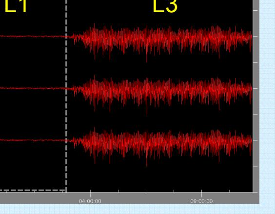
Three channels of acoustic data showing three levels of activity. Each of the three background levels were processed using the Sleeman technique.
