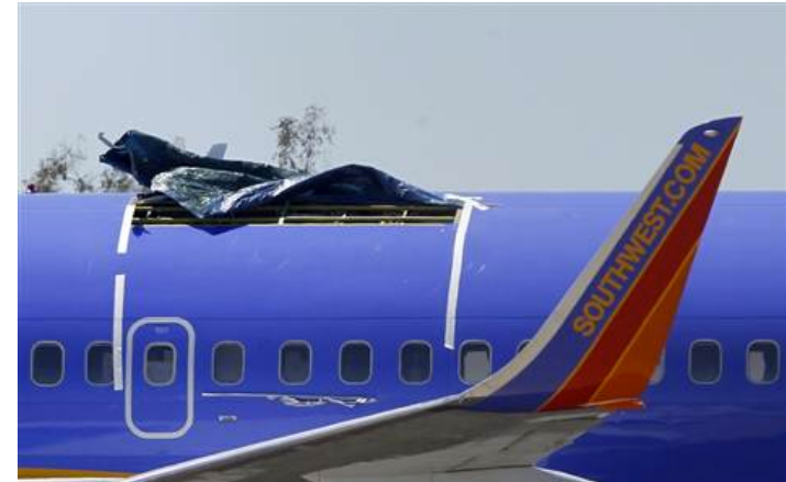
Roof failure (large scale) of Boeing 737 aircraft due to fatigue cracks (small scale). From imechanica.org
