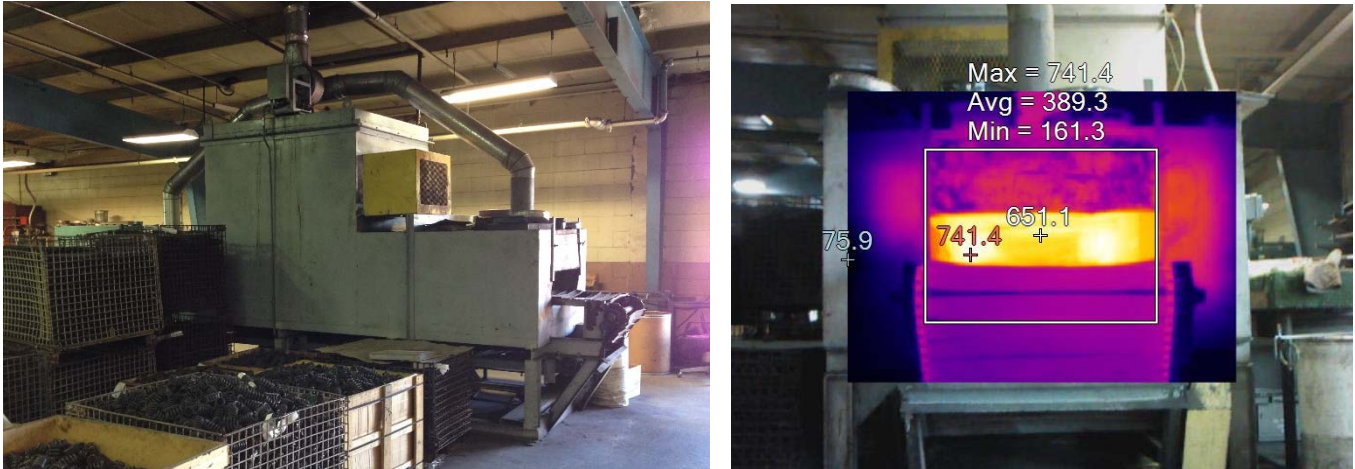
Figure 3 - "Hades" gas fired conveyor oven
