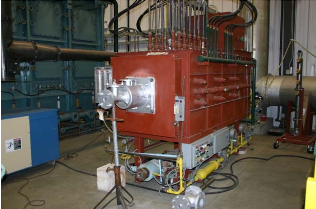
Figure 4. GTI High-Temperature Furnace with Water Cooled Load
