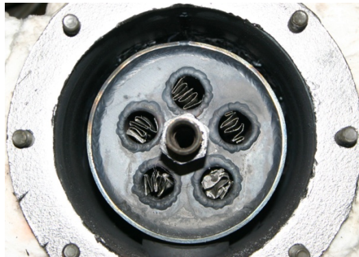
Figure A4. Metal Mesh inside Reformer Tubes
