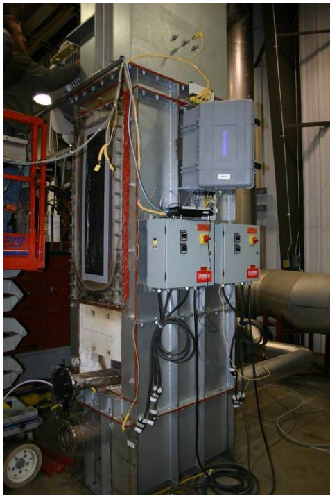
Figure 23. Partially Disassembled Recuperative Reformer at GTI Laboratory
