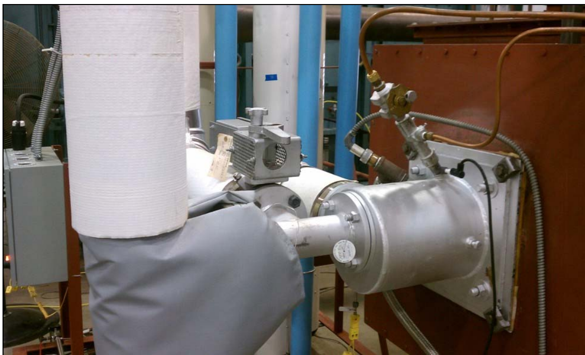
Figure 7. Hot Air Ultra Low NO x Burner by Bloom Engineering Co.
