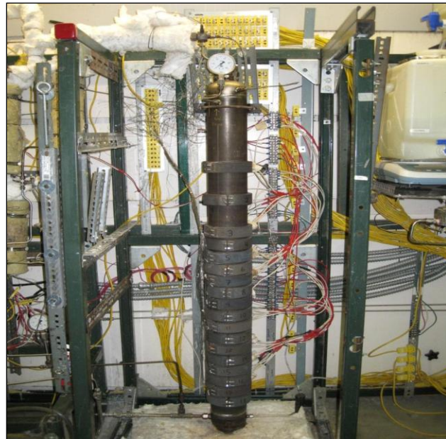
Figure 11. First of Two Forensic Test Reactors at UC-Davis to Examine the Cause of the Methane Reforming Rate (MRR) Fall Off (Unit shown fully instrumented without insulation.)
