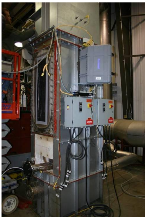
Figure A23. Partially Disassembled Recuperative Reformer at GTI Laboratory
