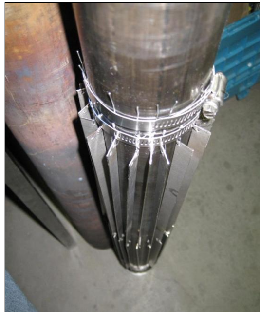
Figure 12. Second of Two Forensic Test Reactors at UC-Davis with High Nickel Alloy Inserts (800H) Installed to Examine the Cause of the Methane Reforming Rate (MRR) Fall Off (Shown in Construction with only Lower Inserts Installed.)
