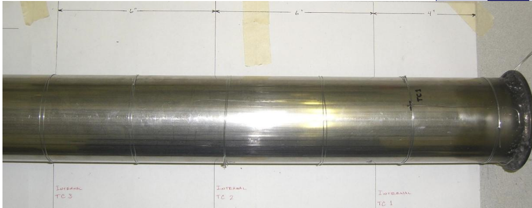
Figure B7: Photograph of thermocouple placement along inner tube. Note, thermocouples are 60° apart axially, 6" apart laterally (Baseline reactor) and 12" apart laterally (Inserts reactor)
