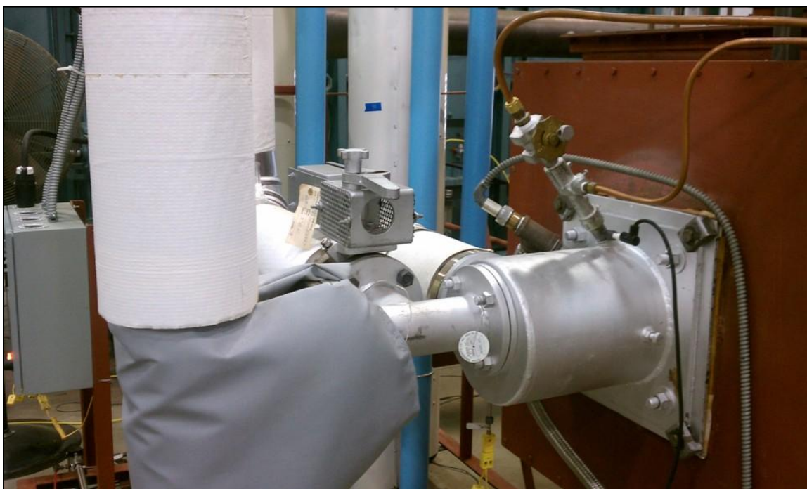
Figure A7. Hot Air Ultra Low NO x Burner by Bloom Engineering Co.
