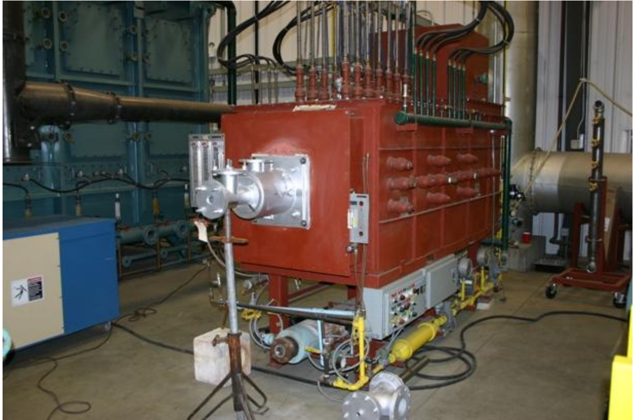
Figure A4. GTI High-Temperature Furnace with Water Cooled Load
