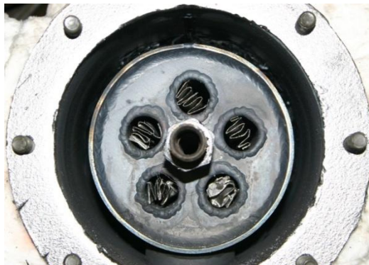
Figure A35. Metal Mesh inside Reformer Tubes
