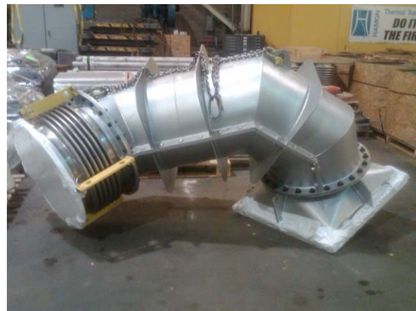
f) Exhaust Connection from Furnace to Reformer
