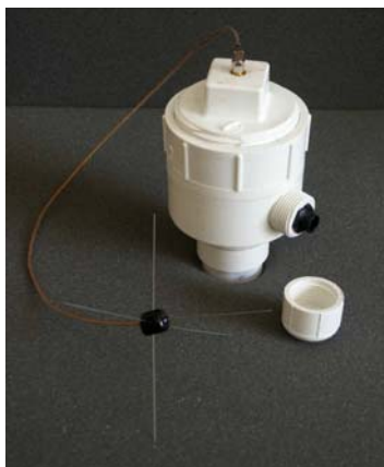
Figure 4. A VPED sensor node with an inconspicuous, ground-mounted antenna gathers data from a variety of sensors and processes information for the cluster node
