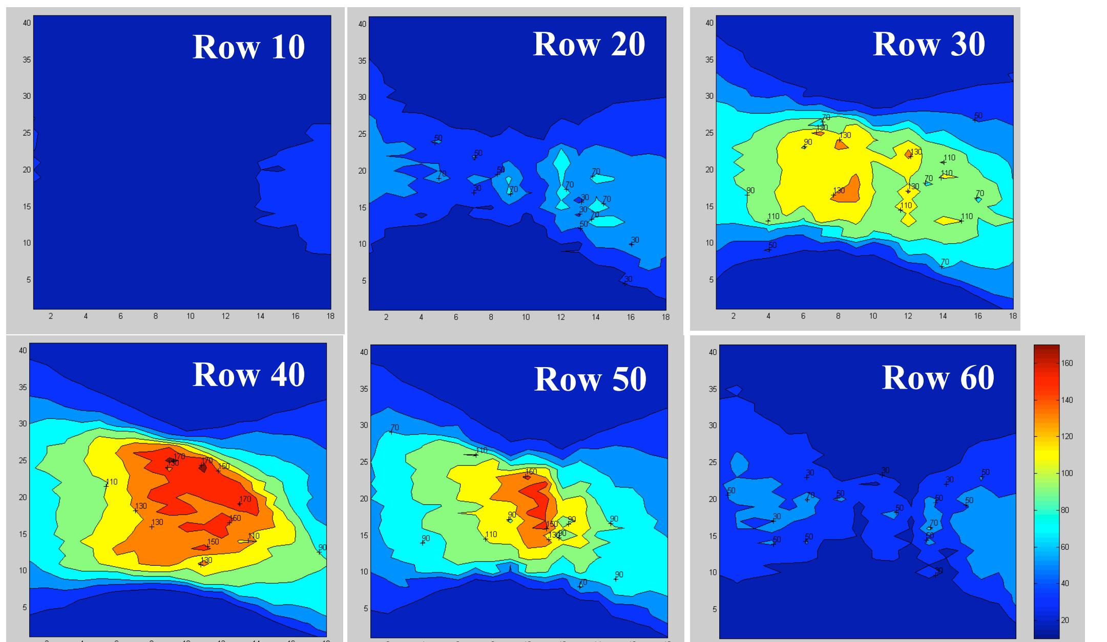
Finally, the practical importance of intensity contour profiling can be seen in the following, where weld penetration vs. defocus data is compared with iso-intensity contour data for a CO<sub>2</sub> laser.
