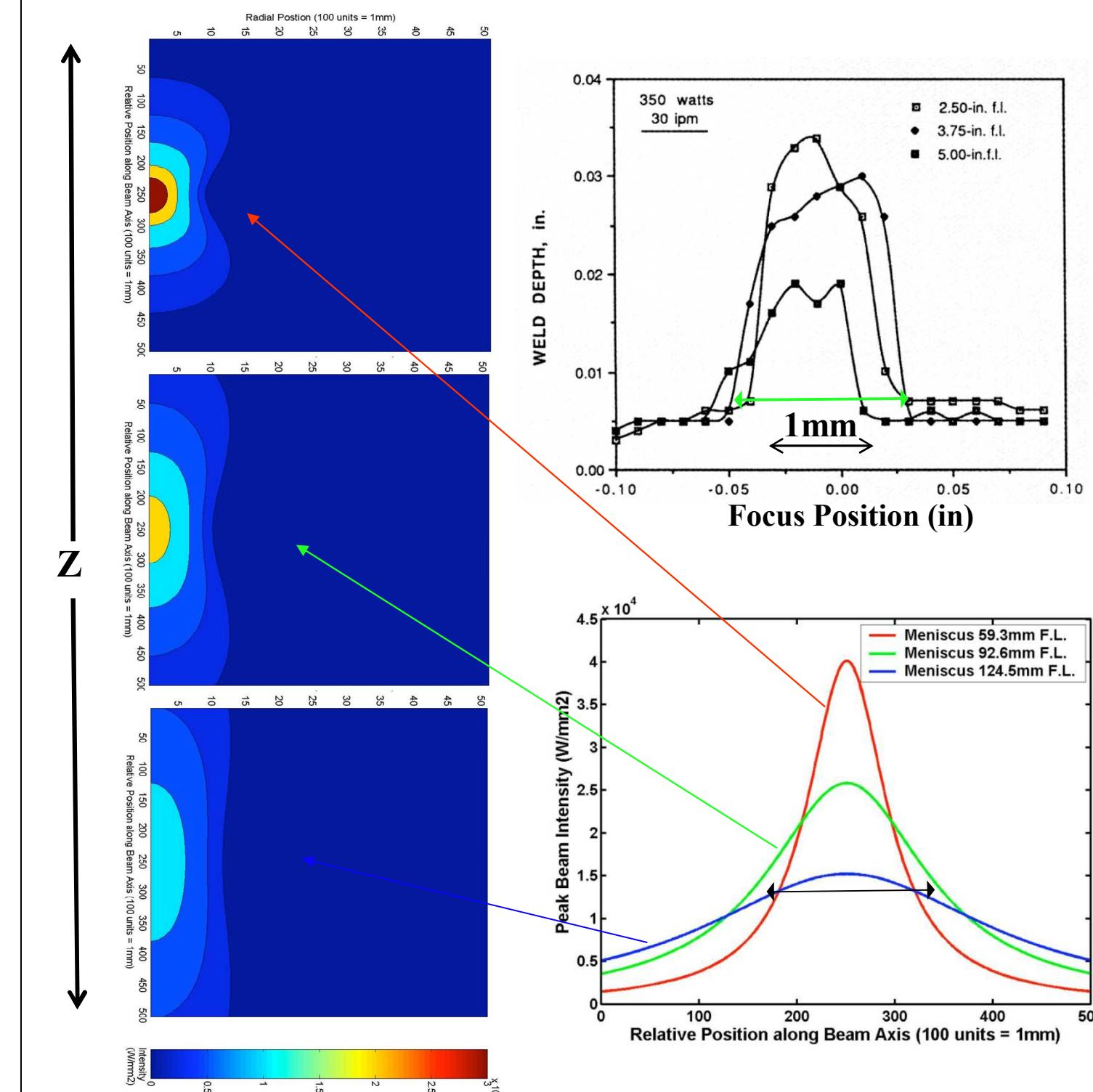
**Schematic conduction and keyhole welds vs. focus position**
