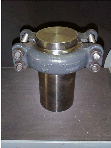
Figure 9. Subscale Vessel Before Testing, After 0.71 Pound Tests, and After Failure
