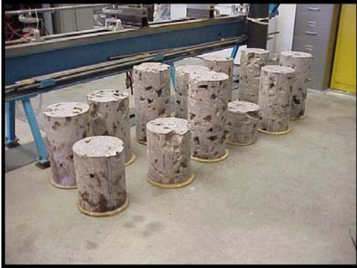
Welded tuff core recovered from YMP
