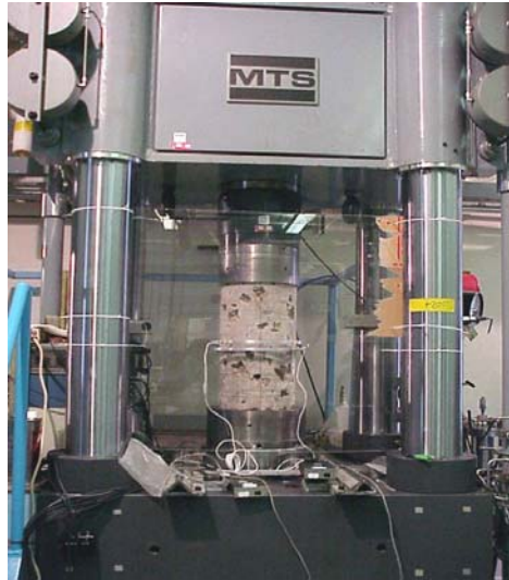
Compression test of lithophysae tuff
