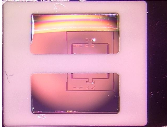
Fig. 7. The first package version used an alumina substrate and incorporated a bar across the sense mass to constrain vertical motions while attempting to allow lateral motions.
