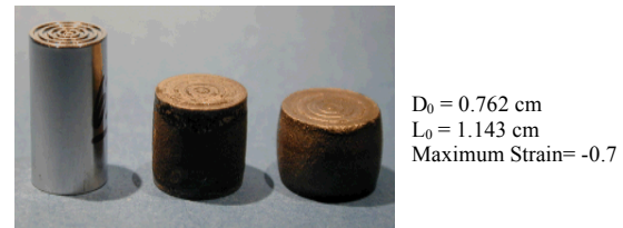
Figure 4: Uniform straining compression specimens
