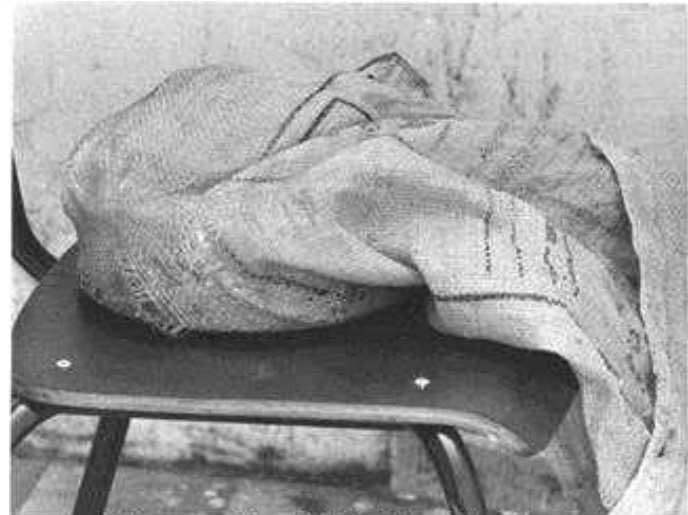
source assembly that was removed from the shielding of the radiation head. It was enveloped by a cloth bagan placed on a chair, which was taken to the corner of the Health Department courtyard. OSEGO.
