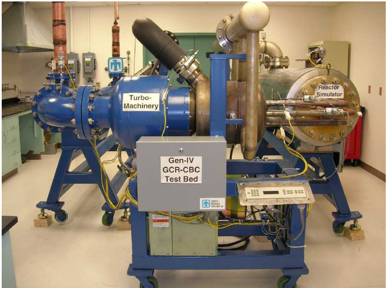
Figure 1: Photo of the Sandia Brayton Loop (SBL-30) installed at Sandia. The water cooled gas chiller is on the left and the electrical heater is on the right. The alternator is inside the blue turbomachinery housing while the compressor, turbine and recuperator are hidden within the stainless steel cylindrical housing and the controllers are mounted to the center frame.
