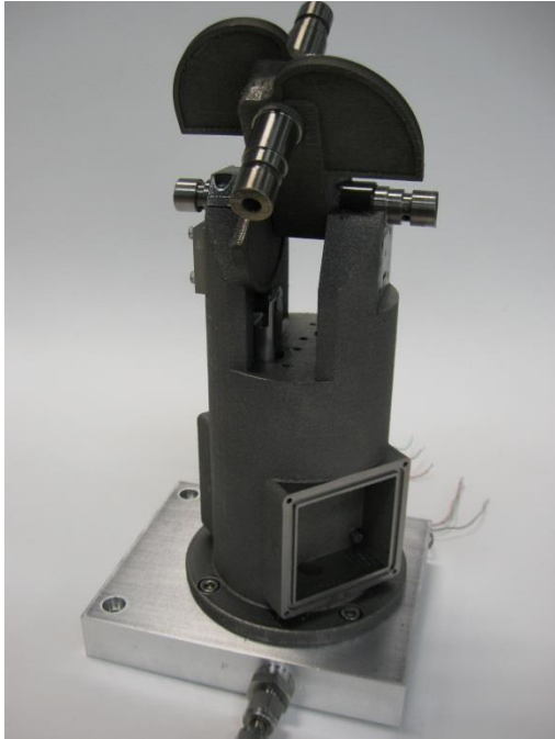
Figure 41. Joint of a robotic arm that embeds hydraulic lines, eliminating external lines for hydraulic fluid and wiring. (used with permission) [185]
