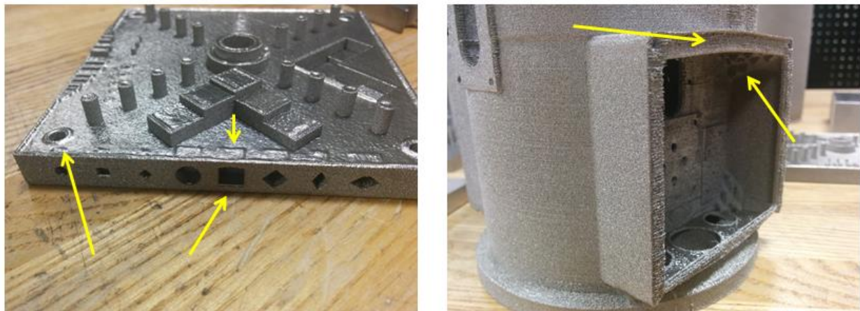
Figure 16. For EBM printed Ti-6Al-4V parts it can be seen that (Left) a NIST test artifact designed to test AM capabilities has overhangs printed in the side of the part. These are intended to test the ability of various machines to print overhangs. Minor swelling can be seen both above the overhang and near a hole on the left side on the top surface. (Right) A complex robotic part shows a slightly deformed overhang, with sintered powder and support stubs left underneath.
