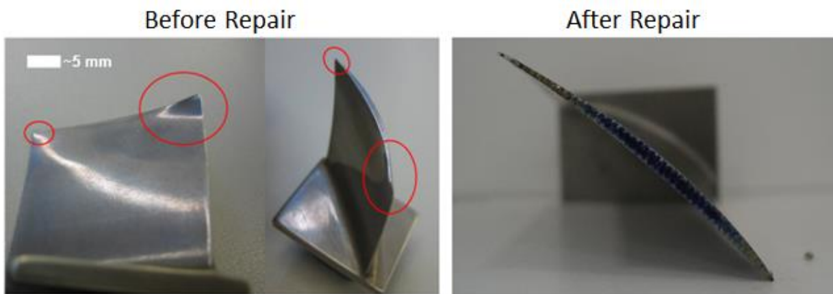
Figure 29. Airfoil repair using a hybrid DED+CNC method. [117]
