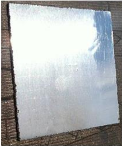
Figure 31. (Left) Bulk metallic glass made in EBM, with amorphous structure [119] and (Right) EBM fabricated Al 2024 impellers on build substrate. [64]
