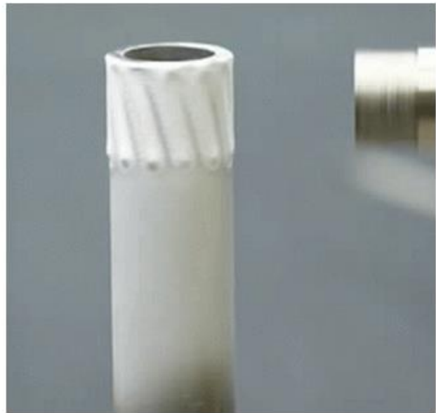
Figure 37. (Left) Operator setting up cold spray AM system, which operates outside of a controlled environment, and (Right) cold spray deposit forming on the tip of a substrate tube that is rotated. [161]
