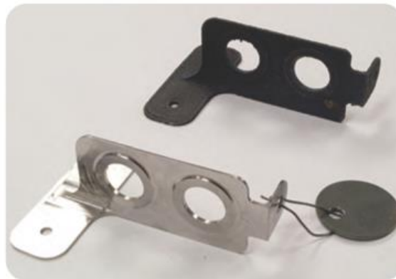
Fig. 7 — As-deposited (top) and post-machined BALD bracket (bottom).
