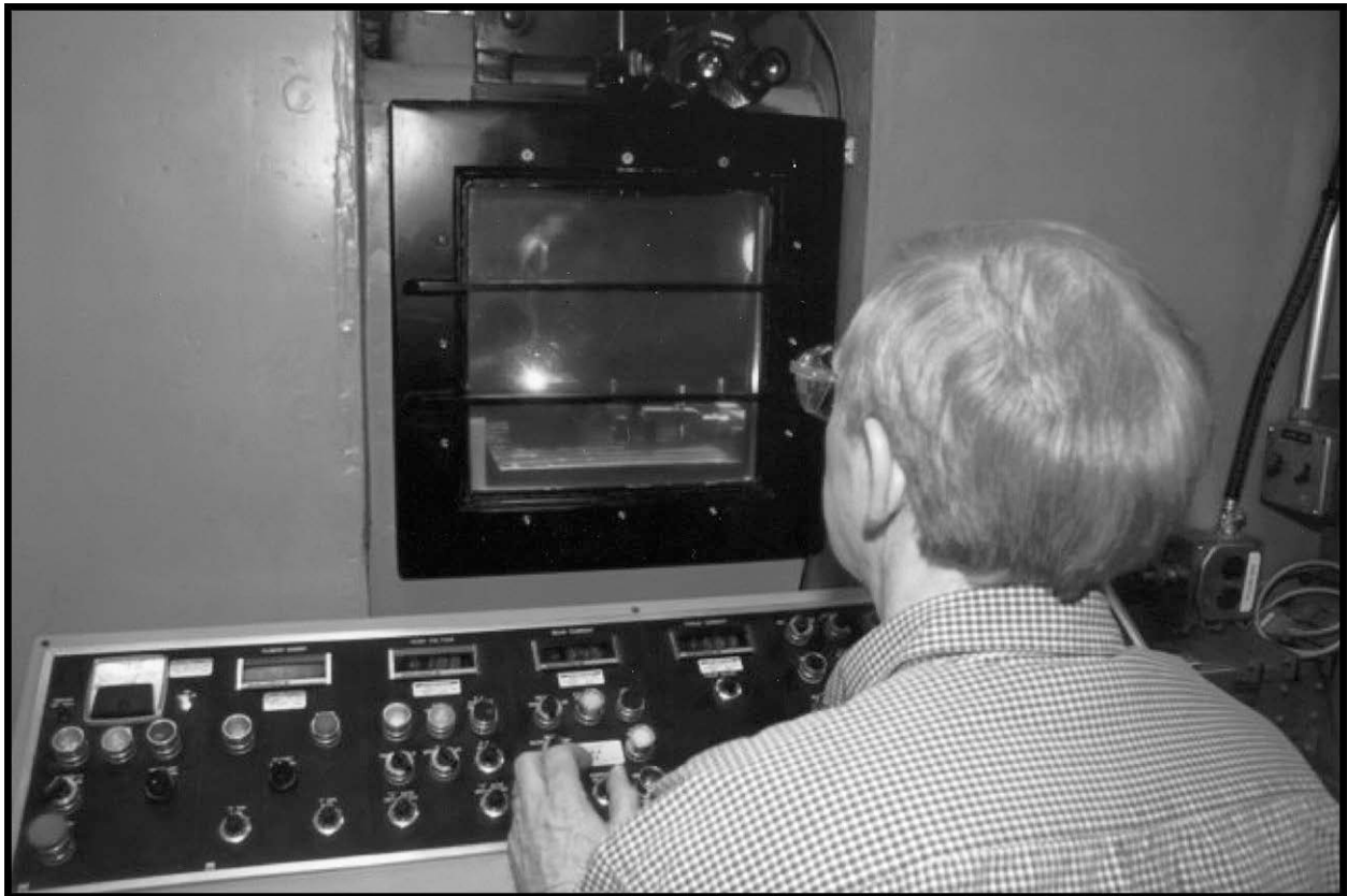
Computer network-controlled laser welding containment
