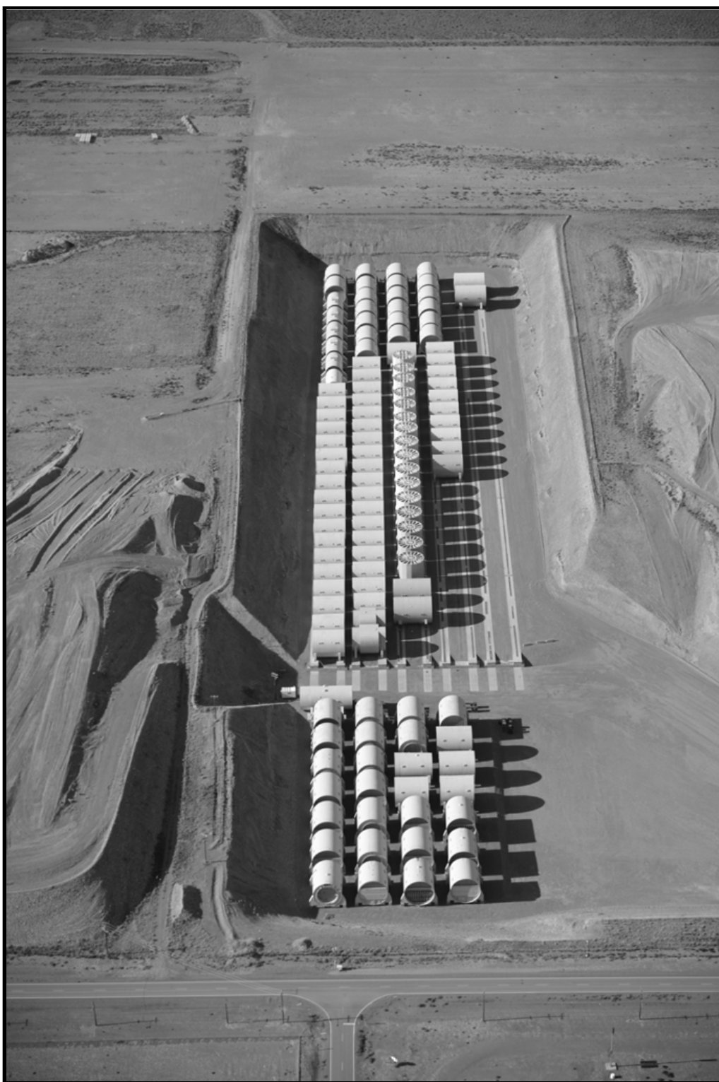
Defueled naval reactor compartments at the Department of Energy's Hanford Site, November 2012
