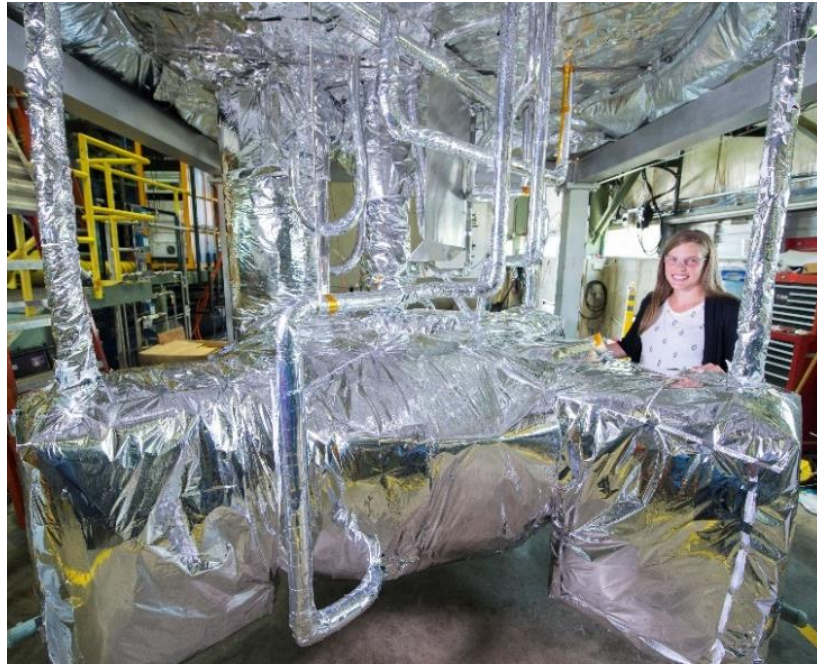
Figure 3: The TS prototype with its custom thermal shield in place.
